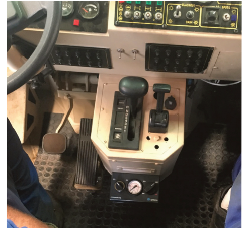
CTIS operating unit in the driver's cabin
