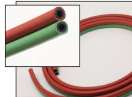
This deadman hose serves as an integral assembly for use as connection to the deadman control valve. Vertically braided textile, twinned 1/4" diameter red and green hose is vulcanized.
