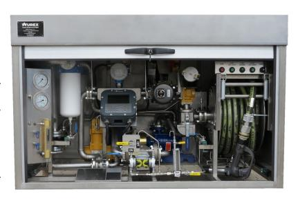
steel enclosure. The refuelling unit is equipped with a stainless steel reel with pressure hose with the length and diameter designed to individual needs of the customer. The unit is also equipped with a filter-monitor or coalescer/separator for removing water in fuel and an additive injector for preventing water crystallization in aviation fuel. The unit has also a connector for drawing fuel samples before and after filtering.
